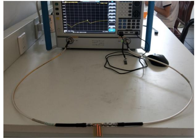
FIGURE 8. Configuration of Ti-NGD circuit prototype experimental setup.
