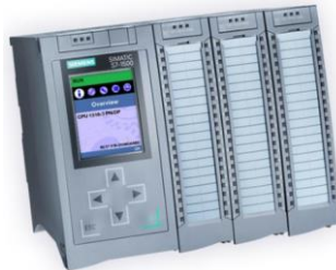
Figure 6: Siemens 1516-3 PN/DP CPU and cards.
