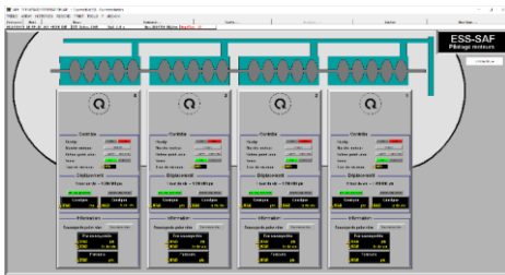
Figure 11: PLC Phytron control view.
