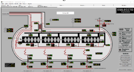
Figure 8: Cryomodule cryogenic PLC.
