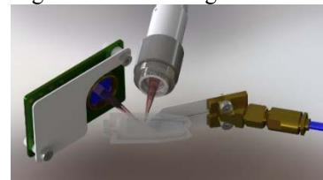
Fig. 2 Design of the laser deflection system for AFM implementation.
