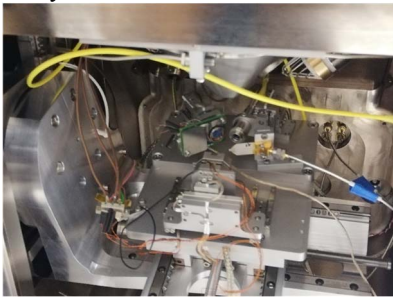
Fig. 4 NSMM integrated in the SEM Tescan® MIRA XMU. The electron gun of the SEM is focused on the probe tip contacting the sample.
