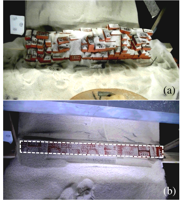
Figure 10: Part of the wall that remained intact during the tilting test. (a) Overturning (width B = 85\text{mm} ) (b) Sliding (width B = 34\text{mm} ).
