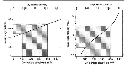
Fig. 4 Porosity of icy particles as derived from the ice-free particle density and the mean nucleus density (left), and refractory-to-ice mass ratio as function of the dry dust particle density and the mean nucleus density (right). The potential parameter ranges based on the COSIMA dust collection are indicated by the shaded areas
