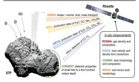
Fig. 1 Schematic overview of measurements by *Rosetta* instruments that inform the parameters needed to derive the dust-to-gas and refractory-to-ice mass ratios of 67P
