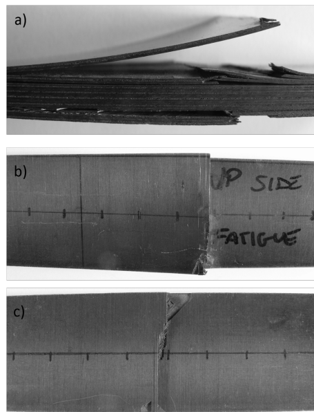
Figure 10: Fatigue test of an impacted sample: Post-mortem profile.
