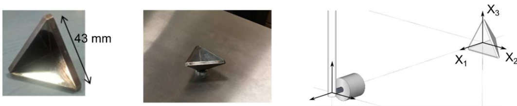
Figure 6: Stainless steel CCR and experimental setup
