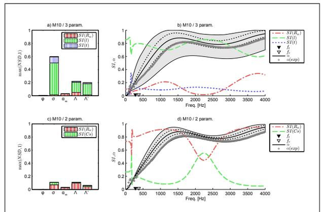
Figure 2. Sensitivity analysis on the foam M10. First line: First-order sensitivity index  $SI$  for macroscopic non-acoustic parameters and associated Normalized Standard Deviation  $NSD$ . Second line: normal incidence sound absorption (bold line: mean value; dotted line: standard deviation; gray area: extremal bounds) and associated first-order sensitivity index  $SI$ . Viscous/inertial and isothermal/adiabatic transition frequencies  $f_v$  and  $f_t$  are also shown on the plots.
