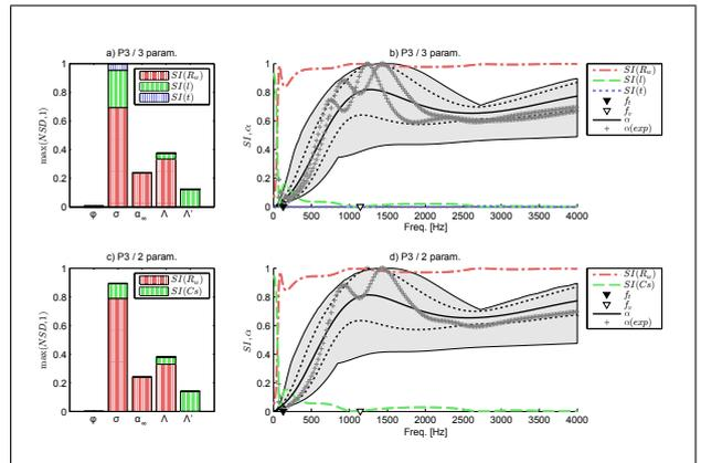
Figure 4. Sensitivity analysis on the foam P3. First line: First-order sensitivity index  $SI$  for macroscopic non-acoustic parameters and associated Normalized Standard Deviation  $NSD$ . Second line: normal incidence sound absorption (bold line: mean value; dotted line: standard deviation; gray area: extremal bounds) and first-order sensitivity index  $SI$ . Viscous/inertial and isothermal/adiabatic transition frequencies  $f_v$  and  $f_t$  are also shown.
