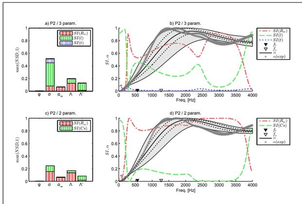
Figure 3. Sensitivity analysis on the foam P2. First line: First-order sensitivity index  $SI$  for macroscopic non-acoustic parameters and associated Normalized Standard Deviation  $NSD$ . Second line: normal incidence sound absorption (bold line: mean value; dotted line: standard deviation; gray area: extremal bounds) and first-order sensitivity index  $SI$ . Viscous/inertial and isothermal/adiabatic transition frequencies  $f_v$  and  $f_t$  are also shown.
