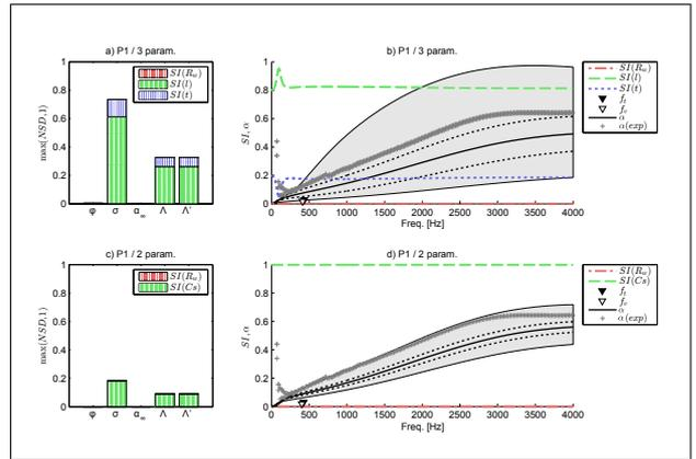
Figure 1. Sensitivity analysis on the foam P1. First line: First-order sensitivity index  $SI$  for macroscopic non-acoustic parameters and associated Normalized Standard Deviation  $NSD$ . Second line: normal incidence sound absorption (bold line: mean value; dotted line: standard deviation; gray area: extremal bounds) and associated first-order sensitivity index  $SI$ . Viscous/inertial and isothermal/adiabatic transition frequencies  $f_v$  and  $f_t$  are also shown on the plots.
