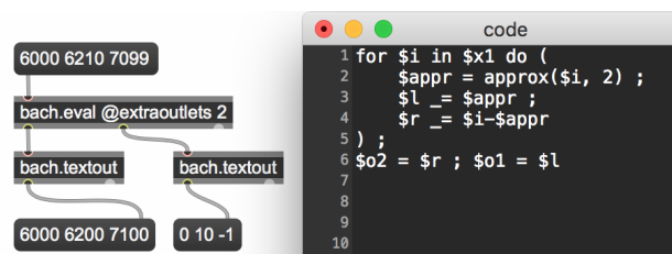
Fig. 7. A snippet of bell code approximating a list of midicents to the nearest semitone, and returning the distances from the semitone grid from a different outlet. Here, the code has been typed in a separate text editing window (shown on the right). The $o1 and $o2 pseudovariabes assign results to the extra outlets declared in the bach.eval object box. The main, rightmost outlet returning the actual result of the computation (which, in this example, is the last term of the sequence defined by the ; operators, that is, the value of the $l variable as passed to the first extra outlet) is left unused here. The language has several other features not shown here, including named and anonymous user-defined functions with a rich calling mechanism.
