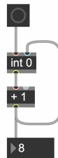
Fig. 1. The typical design of a simple accumulator in Max: the int module stores the current number in a hidden state; when the top button is clicked, the state is output, incremented, and stored in the int module anew. Notice that, as a general rule in Max, the internal state is hidden from the user: at the moment in which the screenshot was taken the internal state had been updated to 8 (as the bottom number displays) although the argument of the int module still shows ‘0’, which represents the initial state. Note also that the functioning here is asynchronous and controlled through hot and cold inlets which differs from the synchronous functioning of the DF accumulator in sect. 2.6
