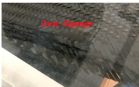
Fig. 8. Forming process for multi-layer reinforcement
