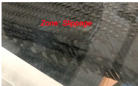
Fig. 8. Forming process for multi-layer reinforcement
