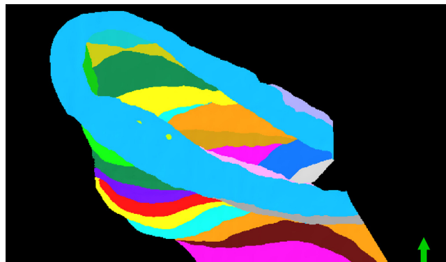
Fig. 10. Zone model of the reservoir under study for the uppermost part of the McMurray Formation. Source: Adapted from Durkin et al. (2017).
