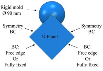
FIGURE 7. Simulation geometry and boundary conditions.
