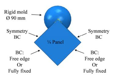
Figure 7. The SRPP preform was modelled using 3D explicit solid elements. Use of 3D solid elements allows full inclusion of transverse shear effects to represent bending, which is of major importance for wrinkling prediction [22]. A mesh size of 1 x 1 mm, and four elements through the thickness were used. Behaviour of SRPP was modelled using a user-defined hyperelastic material (VUMAT), which was developed by Charmetant et al. [33].
