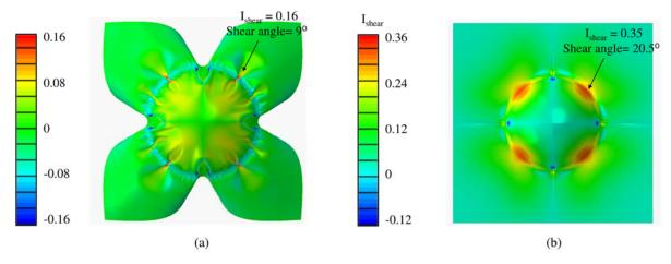
FIGURE 11. In-plane shear angle in simulations with (a) spring-clamping and (b) edge clamping.
