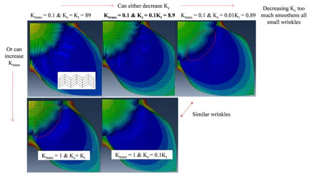
FIGURE 12. Effect of compressive and transverse shear modulus on wrinkle development in spring-clamped SRPP panel. All units are in MPa. The selected combination of  $K_c$  and  $K_{trans}$  is shown in bold.
