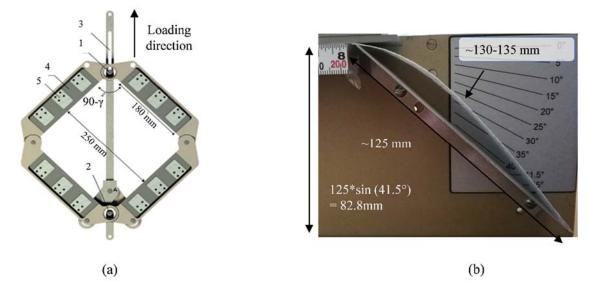
FIGURE 2. (a) KU Leuven picture frame fixture: 1,2 – hinges, 3 – groove, 4 – lip, 5 – plate with screws (adapted from [23]), and (b) Peirce cantilever test fixture with clamped PP textile
