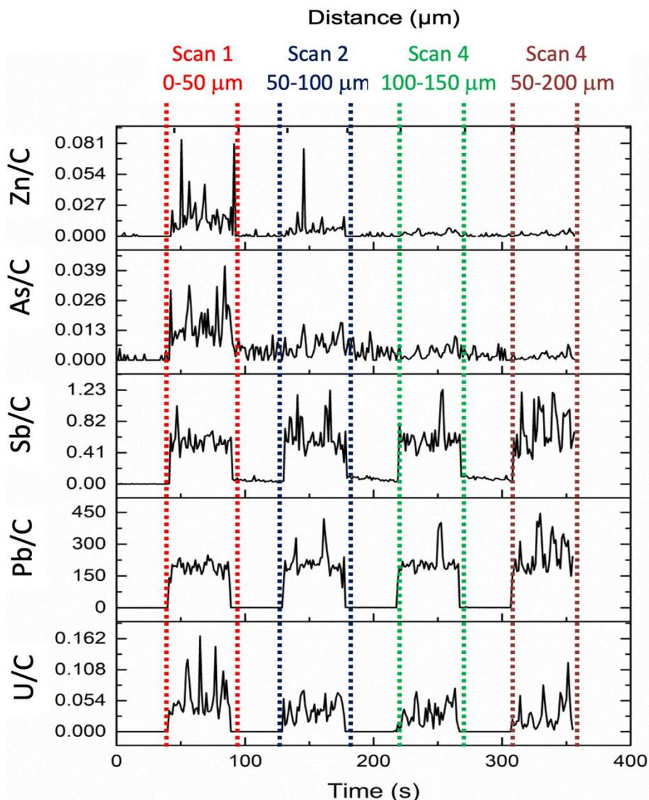
**Figure 1:** Representative results of the LA-ICP-MS analysis of MPG-C polypropylene (PP) microplastic m/z counts (signal intensity) of trace elements ( $^{64}\text{Zn}$ ,  $^{75}\text{As}$ ,  $^{121}\text{Sb}$ ,  $^{208}\text{Pb}$  and  $^{238}\text{U}$ ) relative to the carbon m/z counts for four successive 50  $\mu\text{m}$  depth scans.
