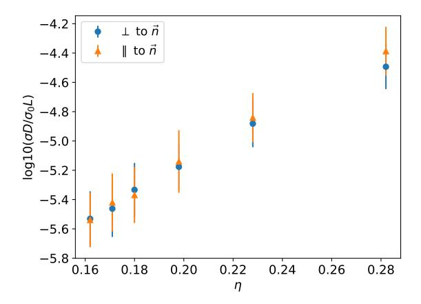
FIG. 7. Conductivity in the nematic phase for  $L/D=20, \lambda=1.2D$ , using the model Eq. 3, as a function of volume fraction.  $\sigma$  measured along the director  $\vec{n}$  of the rods (orange, triangular), compared to  $\sigma$  measured in the orthogonal direction to  $\vec{n}$  (blue, round).
