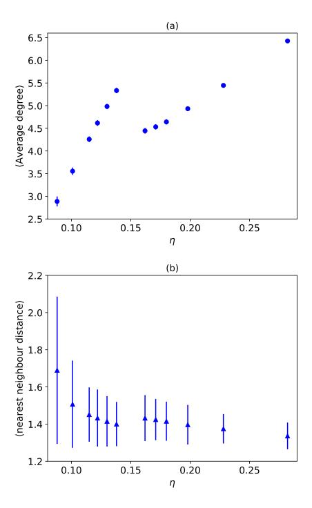
FIG. 3. (a): The average degree of a rod as a function of volume fraction for L/D = 20 and  $\lambda = 1.2D$ . The average degree is simply calculated as twice the size of the edge set divided by the number of nodes in a given network. (b): The mean distance to a rod's nearest neighbour in the largest cluster as a function of volume fraction. In both plots, the error bars are obtained by averaging over all independent realisations of largest clusters per volume fraction.
