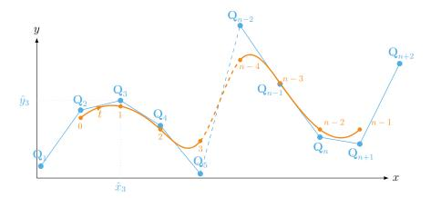
**Figure 2.** parametric curve  $\mathbf{c}(t)$  (----) driven by an arbitrary set of control points (•)
