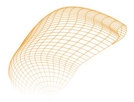
Figure 1. example of a bicubic spline surface
