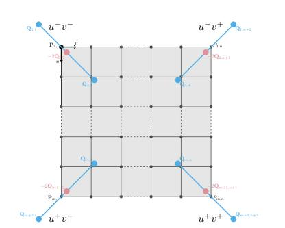
**corner**  $u^+v^+$ : the control point  $\mathbf{Q}_{m+1,n+1}$  is the middle of the segment  $[\mathbf{Q}_{m,n}, \mathbf{Q}_{m+2,n+2}]$ ,
