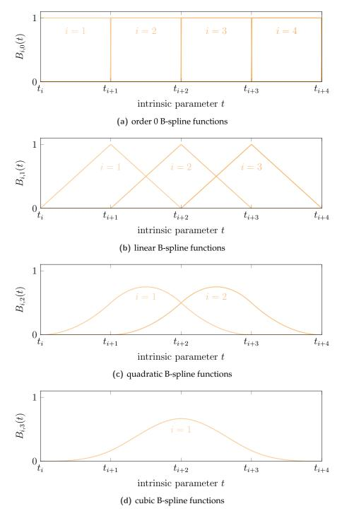
**Figure 3.** B-spline functions with different degree *d* over  $t \in [t_i, t_i + 4]$  and links between *d* degree B-spline functions
