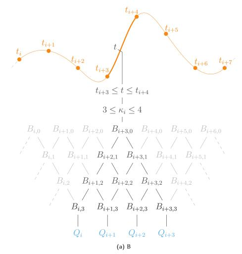
Figure 4. Schematization of the Cox-de-Boor algorythm and links between d degree B-spline functions
