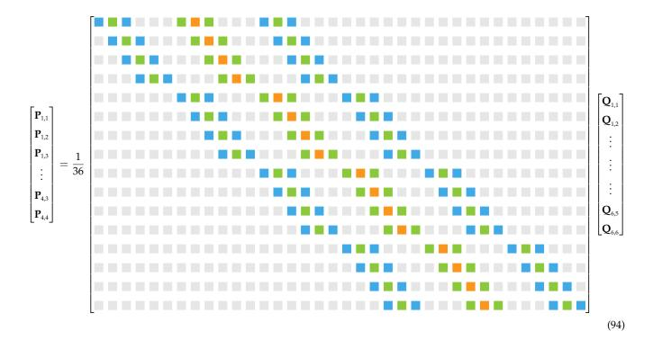
As it stands, the dimensions of vectors **P** and **Q** are not homogeneous and it is not possible to find a unique solution to the problem. Indeed, the length of **P** is still  $m \times n$  while **Q** is  $(m + 2) \times (n + 2)$ . However, adding end condition equations to constrain the shape of the parametric surface will be sufficient to calculate every control point coordinates  $Q_{i,j}$  by inversion.
