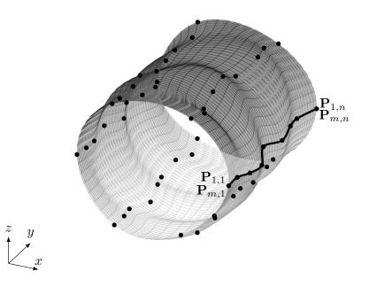
**Figure 19.** closed bicubic parametric surface interpolation on a randomized cylinder with m = 7 and n = 8
