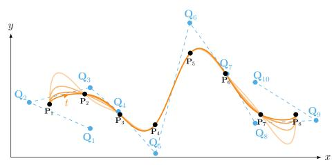
**Figure 7.** parametric cubic spline interpolated on fit knots with different tangent vectors: T = [0, 1] (----), T = [0, 2] (----), T = [0, 4] (----) and T = [0, 8] (-----), control points (•) for T = [0, 1] only
