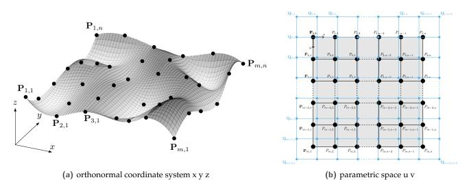
**Figure 10.** bi-spline surface interpoled on fit knots (•)
