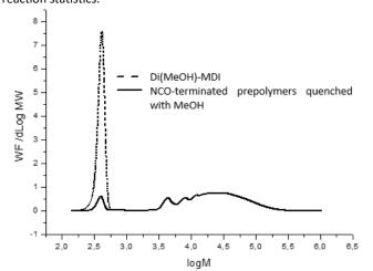
Figure 4. Typical SEC-THF chromatograms of NCO-terminated polyurethane prepolymers quenched with MeOH.
