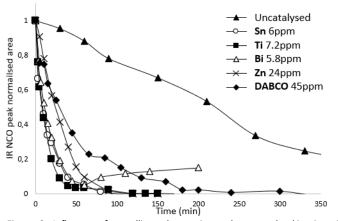
Figure 3. Influence of metallic and organic catalysts on the kinetics of prepolymerization reaction at  $80^{\circ}\text{C}$  determined by FTIR-ATR.
