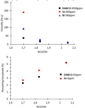
Figure 7. Evolution of remaining isocyanate and NCO-terminated prepolymers viscosity *versus* catalyst nature and NCO/OH ratio. NCO-terminated prepolymer viscosities were measured after one hour of reaction by rheometry.
