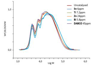
Figure 5. SEC-THF chromatograms of polyurethane NCO-terminated prepolymers, quenched with MeOH, obtained with different catalysts.
