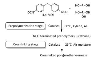
Figure 1. Process for NCO terminated prepolymers and crosslinked polyurethanes.
