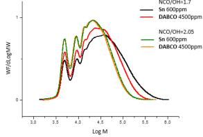
Figure 6. SEC-THF chromatograms of polyurethane prepolymers quenched with MeOH in function of catalyst (nature, amounts) and ratio NCO/OH.
