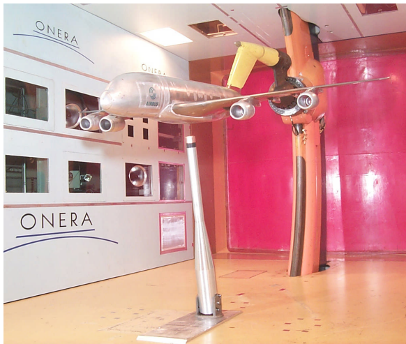
Figure 1: Airbus model during test with dummy strut at F1
