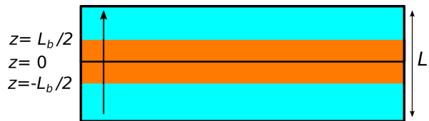
FIG. 3. Geometric parameterization of the system used in the present study, with L = L_b + L_w .
