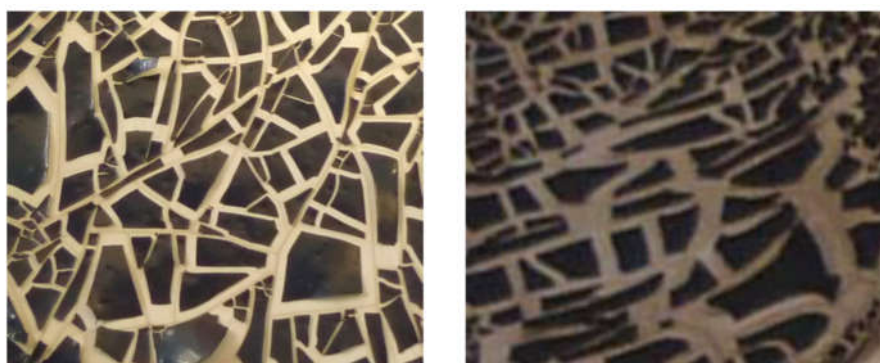
Figure 1. Laboratory sample of asphaltenes extracted from crude oil in n -heptane (left) and n -pentane (right).
