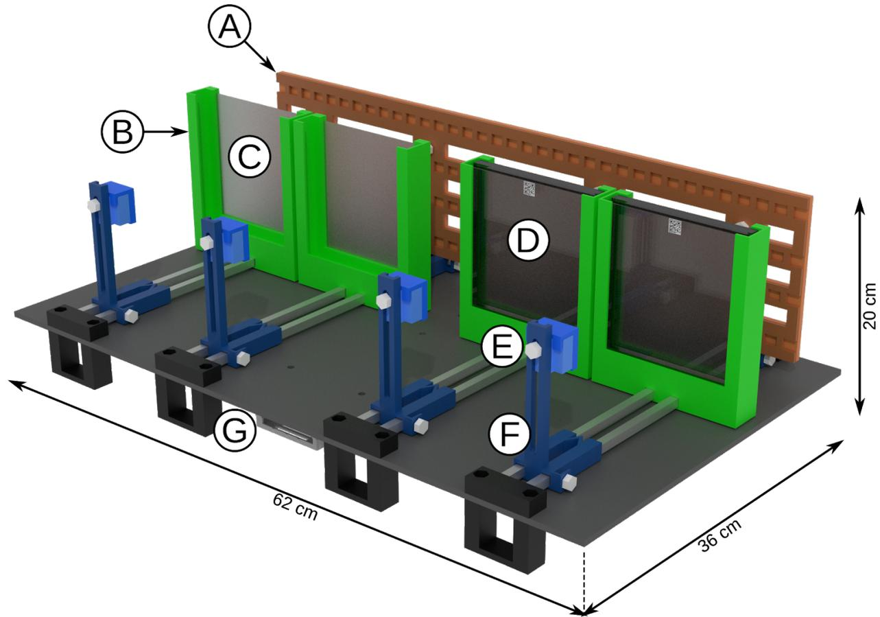
**Supplementary Figure 3. Low-cost device for automatic image acquisition of plant plates.** 3D rendering of a ChronoRoot module. (A) mobile and controlled infrared (IR) backlight (850 nm), (B) mobile plate support, (C) diffusing filter, (D) 12 cm x 12 cm square plate with QR code on the top, (E) Camera case equipped with an IR long pass filter (> 830 nm), (F) mobile camera support, (G) Raspberry Pi computer controlling the module (IR backlight and camera).
