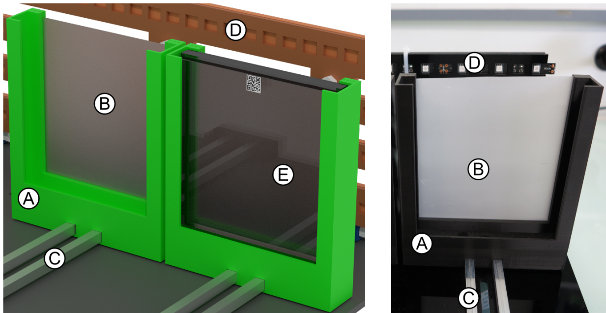
Supplementary Figure 5. Plate support. Annotated 3D rendering (left) and picture (right) of the plate support. The U-shaped plate support (A) carries a diffusion filter at the back (B) allowing an homogeneous near-infrared illumination. Each support moves horizontally on the double axis (C). A classical 12.5 cm x 12.5 cm square plate fit into the plate support (E). Each camera is a regular Raspberry Pi NoIR V2 module (Sony IMX219 8-megapixel sensor) which is able to capture NIR wavelengths in addition to the classical visible spectrum. It is positioned in a box that can be moved vertically on an L-shaped support which can be shifted along the horizontal axis. The focus of the camera is adjusted manually before the start of the experiment by turning the objective lens using the provided crown. To be able to record pictures exclusively from the NIR spectrum, an IR long pass filter (12.5 mm diameter, RG830 Schott AG) can be positioned in front of the camera to exclude light below 830 nm and provide consistent images independently of the lightning of the growth chamber.
