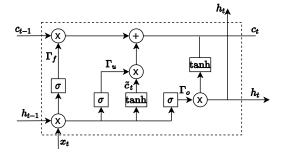
Fig. 2. Cells description of the long short-term memory implementation.
