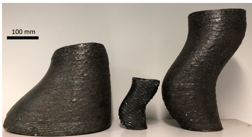
Figure 31 :Parts manufactured with WAAM technology using the continuous path resulting from the CTPP strategy. (Left) Part 2, (Center) Part 1: Height= 16cm, (Right) Part 1 with a scale factor of 2.5.
