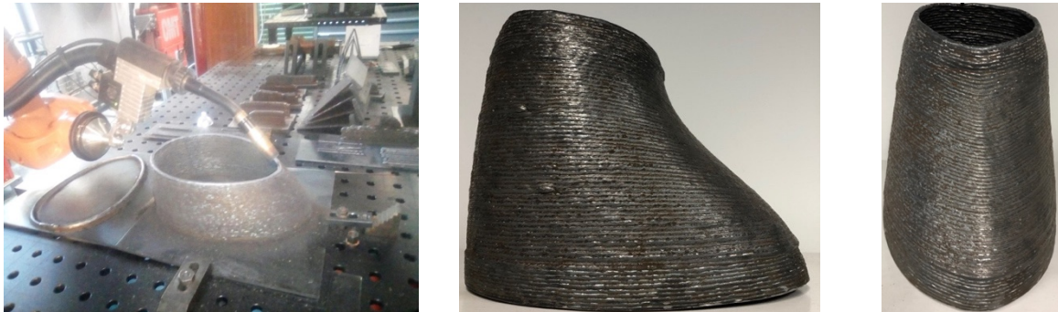
Figure 28 : Different points of view of the open part 2 during the manufacturing process and after, with WAAM technology using CTPP strategy.
