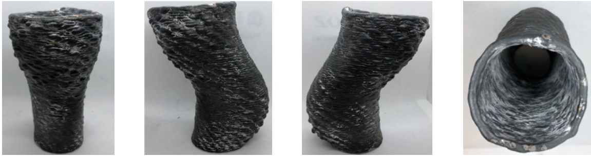
Figure 27 : Different points of view of the open part 1 manufactured with WAAM technology using the continuous path resulting from the CTPP strategy.
