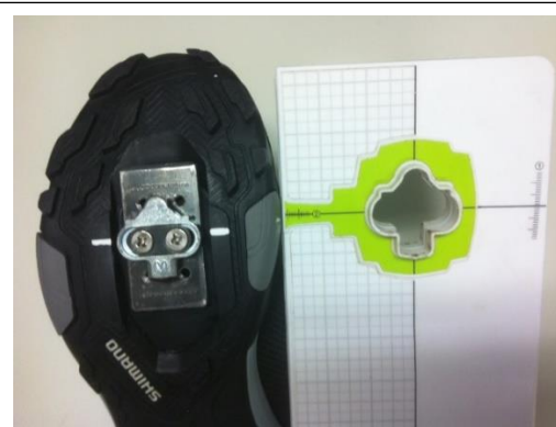
Figure 3: Custom-made system to increase the adjustment range of the cleats.
