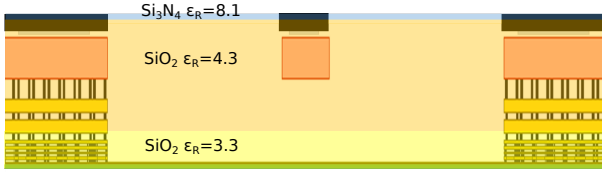
Fig. 1. Cross-sectional side view of a transmission line of fabricated on-wafer TRL calibration kit where dielectric constants levels used in simulation are shown (Run-2). The G-S-G RF pad configuration at M8 is shown in orange, with signal trace in the center. The ground plane is at M1.
