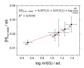
Fig. 4 Calculation of the fraction of H atoms [H], [H]<sub>ToF-SIMS</sub> against log m/I(G) of the impaction ROI. The error bars represent the standard deviation on all acquisitions and include the uncertainties on the Raman spectral data analysis.
