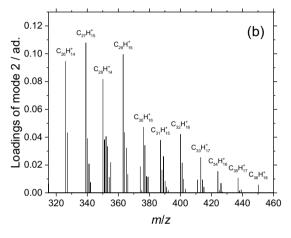
Fig. 5 Criteria used for identifying the correspondences between pairs of ions in mode 1 and individual ions in mode 2. a Number of correspondences found against k for different  $\delta$ . **b** Zoom of the loading plot of PC1 on mode 2. Only the labeled m/z (the highest loading of each group) are selected.
