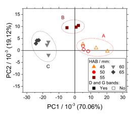
Fig. 2 PC2 vs. PC1 score plot on the impaction ROI showing the three identified data clusters. A (PC1>0, PC2  $\approx$  0): Raman D and G bands have SNR < 3 and no LII is detected, is attributed to condensable gas. B (PC1  $\approx$  0, PC2 > 0): Raman D and G bands have SNR  $\geq$  3 and LII has SNR < 3, is attributed to the transition region. C (PC1 < 0, PC2  $\approx$  0): Raman D and G bands and LII all have SNR  $\geq$  3, is attributed to soot.
