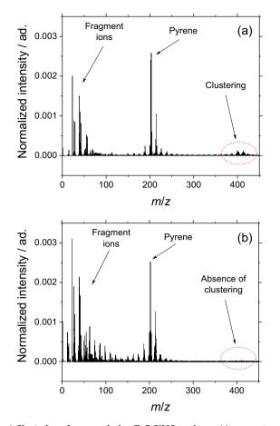
**Fig. 6 Clustering of pyrene during ToF-SIMS analyses.** Mass spectra of (a) pyrene,  $c_{\rm py}=6.03\,\rm M$  and (b) pyrene adsorbed on black carbon  $c_{\rm py}=1.00\times10^{-2}\,\rm M$  to simulate soot. Several fragment ions can be identified on the left side of the mass spectra. The weak signals at m/z 400-420 in panel (a) are attributed to clustering reactions.
