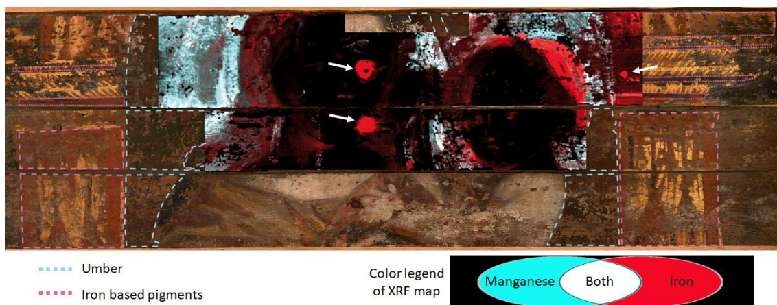
FIGURE 12 X-ray fluorescence (XRF) false color mapping. The iron ( K\alpha lines) is in red, manganese ( K\alpha lines) in blue and mix of both in white. Based on data extrapolated from false color principal components analysis (PCA) composite images, dotted pink lines highlight iron based pigments (hair and architectural columns), whereas dotted blue lines underline umber (the background).
