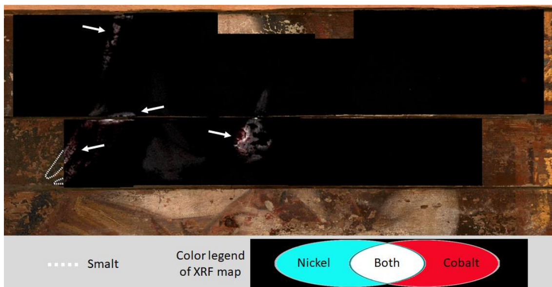
FIGURE 21 X-ray fluorescence (XRF) map in false color, cobalt ( K\alpha lines) appears in red, nickel ( K\alpha lines) is in blue and the mix of both in white. Based on data extrapolated from false color principal components analysis (PCA) composite images, the dotted white line and the white arrows show the area with cobalt blue.
