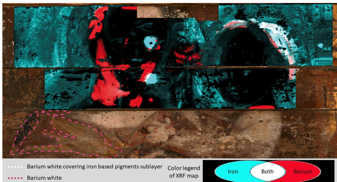
FIGURE 24 False color C-ray fluorescence (XRF) map. Barium ( L\alpha lines) is in red, iron ( K\alpha lines) is in blue and mix of both in white. The red and white areas represent restorations with barium white. Based on data extrapolated from false color principal components analysis (PCA) composite images, the dotted white lines underline the restored part of the hair of the Child and the dotted pink lines are the clothes of the Virgin.
