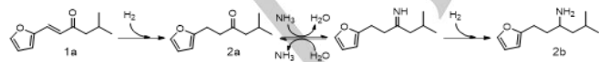
Scheme 2. Reaction pathway for the catalytic conversion of 1a into the furanic amine 2b over Ru/C.
