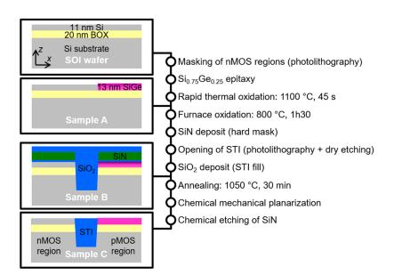
**FIG. 1.** Flow chart summarizing the fabrication of the samples. The schematic of each sample is detailed.
