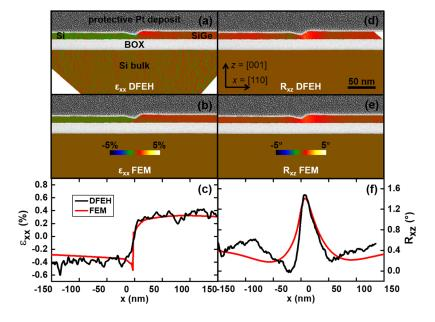
FIG. 2. In-plane strain maps of sample A measured by (a) DFEH and (b) simulated by FEM. (c) In-plane strain profiles extracted within the thin layer. Rotation maps of sample A measured by (d) DFEH and (e) simulated by the FBM model. (f) Rotation profiles extracted within the thin layer. The colored strain and rotation maps originating from the crystalline parts of the sample are encrusted in the bright-field TEM images showing the amorphous regions in gray, to help the reader.
