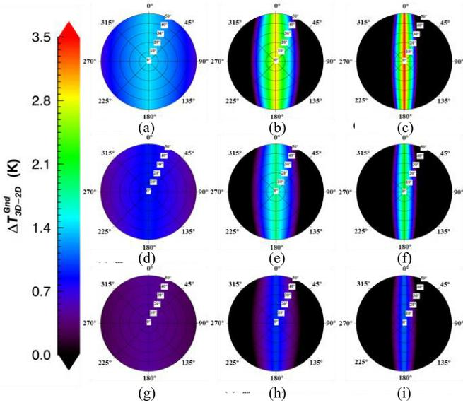
Fig. 4. Magnitude of the impact of 3-D structures and their radiation on ground TIR measurements over a street canyon under different combinations of road emissivity and  $H/W$  on the basis of (30), (34), and (37). Additional parameters have been set as the default values listed in Table I.
