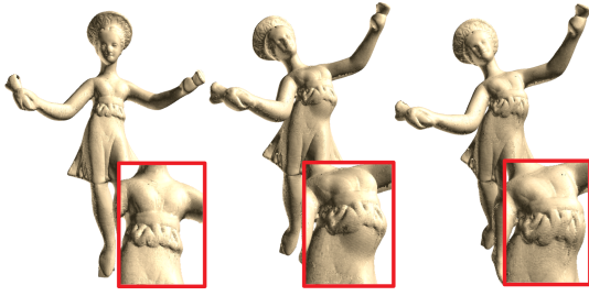
Figure 5: Heightfield skinning. From left to right: original point set; pose change with direct point set skinning; pose change with heightfield skinning.
