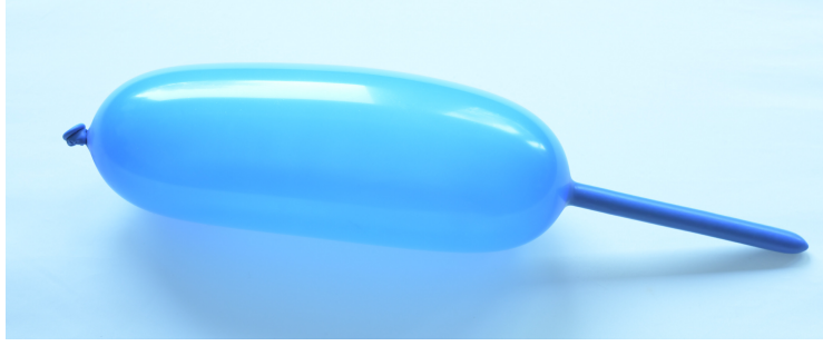
FIG. 4: An inflated tubular balloon is an example of phase separation in a 1D system: a portion with very large expansion of the diameter (on the left of the balloon) coexists with a portion in a phase with rather small deformation (right side of the balloon).
