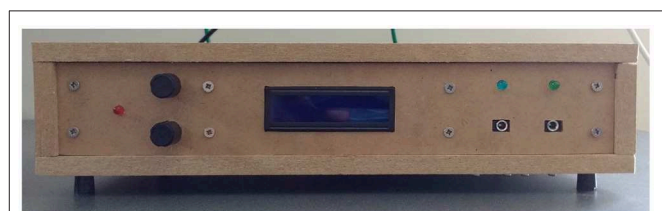
FIGURE 7 | Front panel and user interface for the device. From left to right, the elements are: red power indicator light, rotary encoder adjustment knobs, LCD, photodiode, and microphone input jacks with corresponding blue and green indicator lights.
