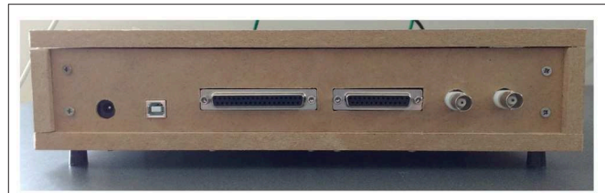
FIGURE 5 | The back panel of the device. From left to right, the connections are: 2.1 mm barrel connector for the power supply, USB port for updating the software, DB37, DB25, photodiode output BNC connector, and microphone output BNC connector.
