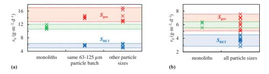
Fig. 2. Comparison of r<sub>0</sub> measurements on (a) ISG glass and (b) Type S glass. r<sub>0</sub> measured on glass particles are normalized to S<sub>geo</sub> or S<sub>BET</sub>.
