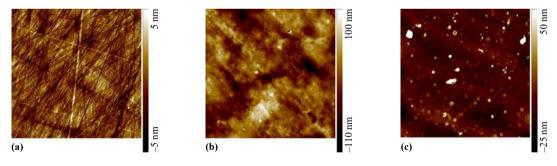
Fig. 1. 10  $\mu$ m x 10  $\mu$ m AFM images of (a) ISG glass polished monolith ( $\Delta S = 1.0\%$ ); (b) 500-750  $\mu$ m Type S glass bead ( $\Delta S = 4.6\%$ ); (c) 63-125  $\mu$ m ISG glass crushed particle ( $\Delta S = 1.1\%$ ).
