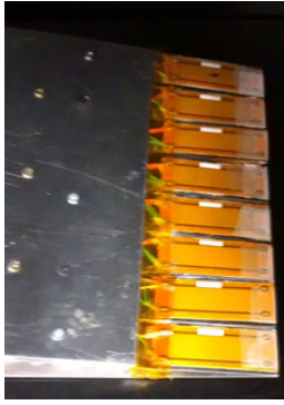
Figure 3: Series of piezo-electric patches installed in the wing's trailing-edge
