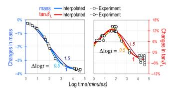
Figure 2: Smoothing and interpolation of experimental data, illustrated for changes in mass (left) and in damping coefficient  $tan\delta_1$  (right) through time. Interpolation is shown for different values of the standard deviation of the Gaussian kernel (Alogt). The value chosen for the analysis (Δlogt = 1) is a trade-off to smooth experimental noise with only slight flattening of curves. Example: from 65 to 35% RH, protocol H, spruce in L direction.
