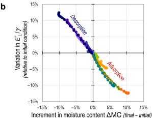
**Figure 5:** Variations (relative to initial value, after a step-change in RH) in (a) damping  $\tan \delta$  and (b) specific modulus of elasticity  $E'/\gamma$ , for spruce in longitudinal direction, as a function of increment in MC.
