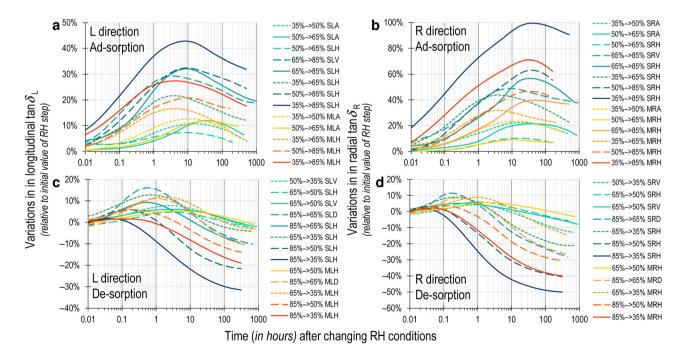
Figure 4: Variations (relative to value in initial condition) in damping coefficient tanδ through time after step-change in RH, for all tested samples and RH-steps. (a, b) ad-sorption, (c, d) de-sorption, (a, c) longitudinal (L) and (b, d) radial (R) directions. RH steps, species, material direction, and protocol (Figure 1) are indicated in the legend. Turquoise-to-blue curves: spruce, yellow-to-red curves: maple.
