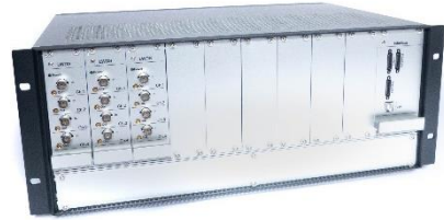
Figure 2: Up to 36 PZT channels simultaneously emitting or receiving signals with 1µs selective commutation
