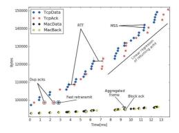
Fig. 8: TCP and MAC sender side-time/sequence plot
