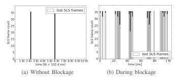
Fig. 6: Correlation between occurrence of blockage and number of lost SLS frames at client-side. During blockage, a large number – 864 (36x24) – of SLS frames is transmitted during a single Beacon Interval (BI), providing ample samples for reliable blockage detection.
