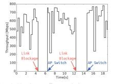
Fig. 4: Handover effect on link connectivity
