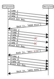
Fig. 7: Link layer retransmission on error
