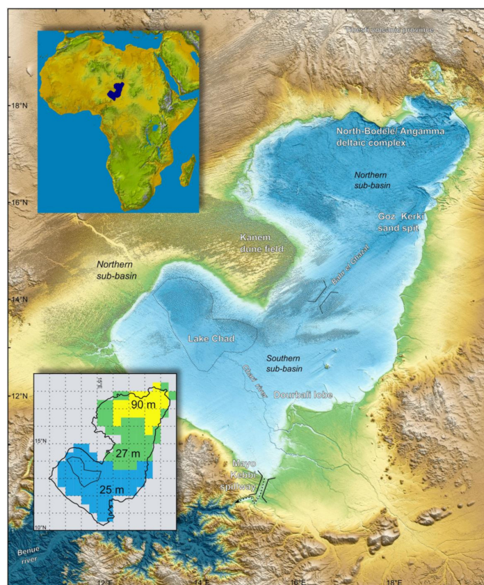
Figure 1. Digital elevation model (SRTM3) of the Chad Basin showing the paleo-extent of Megalake Chad (in light blue), the outline of the Lake Chad in the 1960s (dotted line), and the location of the main areas mentioned in the main text (for more details see [29,40–42]). Upper-left inset: extent of Megalake Chad compared to Africa. Lower-left inset: approximation used to compute the hydro-isostatic rebound related to the drying up of the MLC (the black line represent the 325 m-level line; note the three distinct sub-divisions used to model the load, values refers to their respective mean depths).
