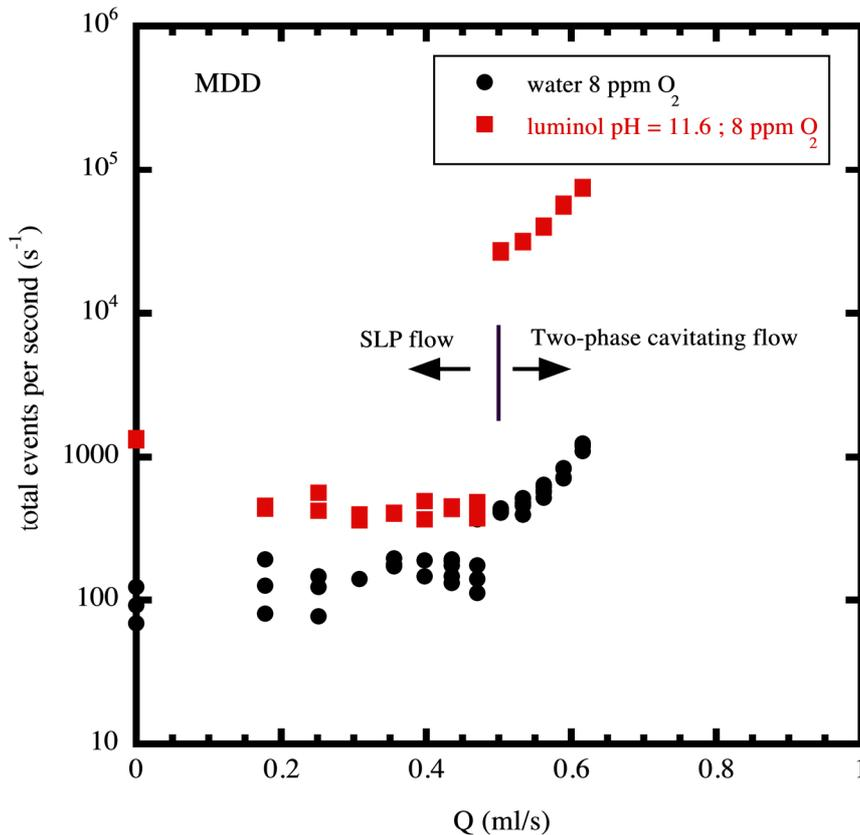
**Figure 8.** Total rate of photons emitted by luminescence and chemiluminescence from the microdiaphragm device. SLP : single liquid phase.
