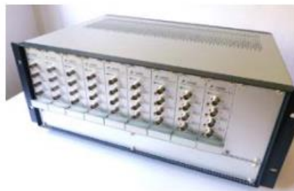
Figure 2 : Up to 36 PZT channels simultaneously emitting or receiving signals with 1 \mu s selective commutation
