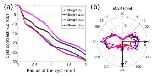
**Figure 8.** (a) Cyst contrast in dB, *CcdB*, computed for LSF of Thread 2 as a function of the radius of the cyst. The curves correspond to the different angular sampling periods and transmit modes; (b) polar representation of the anisotropic cystic resolution aCyR assessed on the LSF of Thread 2 for the different angular sampling periods and transmit modes.
