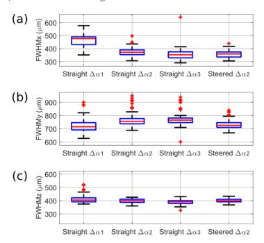
**Figure 6.** Boxplots of the FWHM along the three axes of the coordinate system: (a) FWHMx, (b) FWHMy, (c) FWHMz. The median value is shown with the red line. The box indicates the IQR values and the outliers are shown with red crosses. In abscissa, the scanning name corresponds to the type of transmit and the angular period. The angular periods are  $\Delta\alpha_1 \approx 8^\circ$ ,  $\Delta\alpha_2 \approx 4^\circ$  and  $\Delta\alpha_3 \approx 2^\circ$ .
