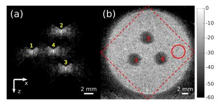
**Figure 7.** (a) xz-image of Ph3 (20 mm x 20 mm); (b) xz-image of Ph2 (30 mm x 30 mm). Both xz-images are at y = 0 and centered on x = 0 et z = 25 mm. They correspond to acquisitions performed in straight transmit at  $\Delta \alpha_2$  with L = 30mm. Numbers identify the threads (a) and holes (b), respectively. The speckle zone considered to calculate the image contrast is designated with a red circle in (b).
