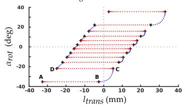
**Figure 3**. Successive motor positions for a rotate-translate scan with the angular sampling period  $\Delta \alpha z \approx 4^{\circ}$ . Positions used for reconstruction are shown with red markers. The black crosses represent targeted endpoints for the motor trajectories. The first four endpoints are notated A, B, C and D.
