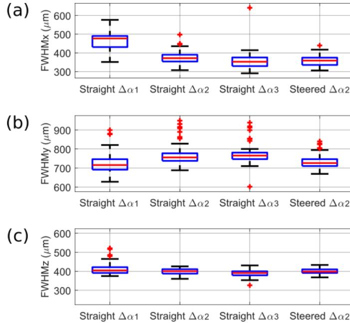
**Figure 6.** Boxplots of the FWHM along the three axes of the coordinate system: (a) FWHM<sub>x</sub>, (b) FWHM<sub>y</sub>, (c) FWHM<sub>z</sub>. The median value is shown with the red line. The box indicates the IQR values and the outliers are shown with red crosses. In abscissa, the scanning name corresponds to the type of transmit and the angular period. The angular periods are  $\Delta\alpha_1 \approx 8^\circ$ ,  $\Delta\alpha_2 \approx 4^\circ$  and  $\Delta\alpha_3 \approx 2^\circ$ .
