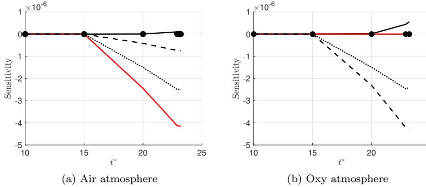
Fig. 8: Evolution of free stream sensitivities, extracted for burning rate,  $\dot{M}$ , as QoI, for air and oxy atmospheres: —,  $N_2^\infty$ ; —,  $T^\infty$ ; - - -,  $CO_2^\infty$ ; ···,  $O_2^\infty$ ; •,  $CO^\infty$ .
