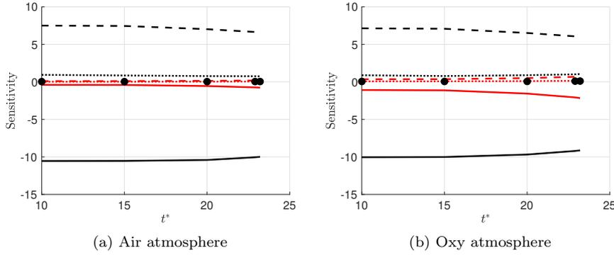
Fig. 5: Evolution of sensitivities, extracted for burning rate,  $\dot{M}$ , as QoI, for air and oxy atmospheres: —,  $E_2$ ; - - -,  $n_2$ ; ···,  $A_2$ ; —,  $E_1$ ; - - -,  $n_1$ ; ···,  $A_1$ ; •,  $\lambda_g$ .
