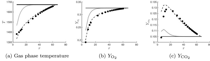
Fig. 1: Evolution of spatial distribution of temperature, oxygen mass fraction ( $Y_{O_2}$ ), and carbon dioxide mass fraction ( $Y_{CO_2}$ ) in the spatial domain, for air atmosphere: —, ( $t^* = 10^{-10}$ );  $\cdots$ , ( $t^* = 18.85$ ); — —, ( $t^* = 22.14$ );  $\bullet$ , ( $t^* = 27$ ).
