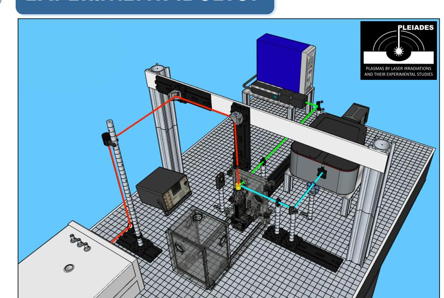
The **first pulse** (1064 nm, 30 ps, 14 mJ) is focused to produce a plasma. The **second** pulse (512 nm, 6 ns, 65 mJ) is focused in this plasma with a temporal shift of  $\Delta t$ . Heated plasma's radiation is collected on a third optical axis to be analysed by our SCT-320 spectrometer.
