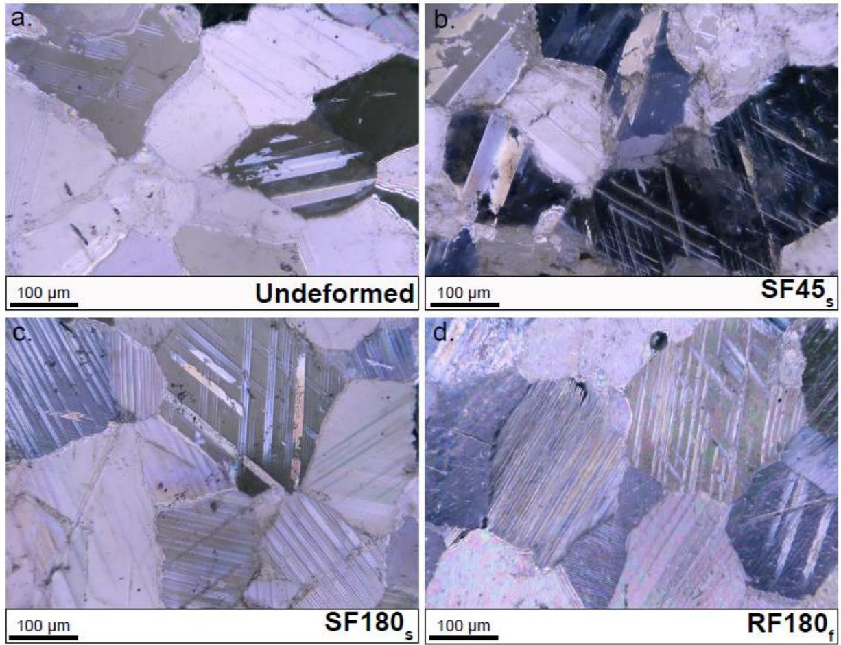
**Figure 11. Thin sections.** Thin sections of the undeformed Carrara marble (a), (b) of the smooth sample deformed at 45 at slow loading rates (SF45<sub>s</sub>), (c) of smooth sample deformed at 180 MPa at slow loading rates (SF180<sub>s</sub>) and (d) of a rough sample deformed at 180 MPa at fast loading rates (RF180<sub>f</sub>). The thickness of twins seems to decrease with confining pressure, so that their density increase. The presence of intra-grains twins is larger for rough conditions.
