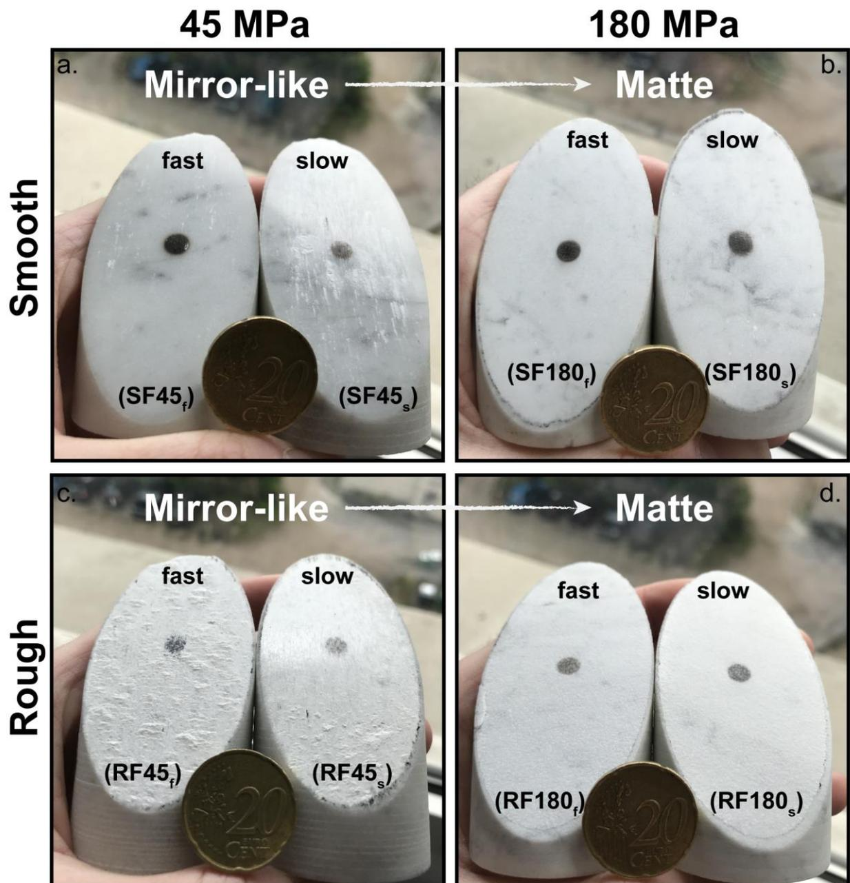
**Figure 5. Macroscopic pictures of the footwall of the fault after experiments.** A transition from mirror-like (SF45<sub>f</sub>, SF45<sub>s</sub>, RF45<sub>f</sub>, RF45<sub>s</sub>) to matte surfaces (SF180<sub>f</sub>, SF180<sub>s</sub>, RF180<sub>f</sub>, RF180<sub>s</sub>) seems systematic after experiments with increasing confining pressure, whatever the loading rates or the initial roughness of the fault, either smooth (a and b) or rough (c and d). Scale is a quarter of euro coin.
