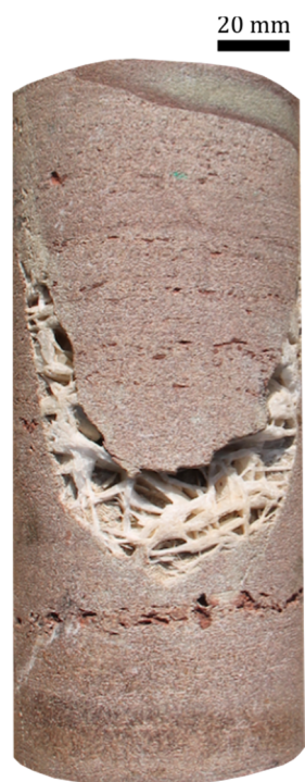
47 Figure 1. Photograph of a section of 78 mm-diameter, cylindrical sandstone core (from the Buntsandstein unit) taken 48 from the Soultz-sous-Forêts (France) EPS-1 exploration borehole, a borehole fully cored from a depth of 930 m to a 49 depth of 2227 m in 1990-1991 (see 5-7 for information on the Soultz-sous-Forêts drilling project). The sandstone core, 50 red/green in color, was taken from a depth of 1374 m and contains a 1-2 cm-wide fracture (in the center of the core). The 51 fracture is partially filled with barite crystals (white in color) that have precipitated from the circulating geothermal 52 fluids.
