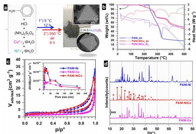
**Figure 1.** (a) Sketch of the used strategy for the synthesis of nickel cobaltite self-supported onto a matrix made of C, N, S, Ni and Co. (b) TGA (left y-axis, solid lines) and DSC (right y-axis, dotted lines) curves in an aluminum crucible in the range of 25-500 °C ( $5\text{ °C min}^{-1}$ ,  $100\text{ mL min}^{-1}$ ). (c)  $N_2$  adsorption-desorption isotherms and the corresponding pore size (diameter) distribution. (d) XRD patterns, see text for details.
