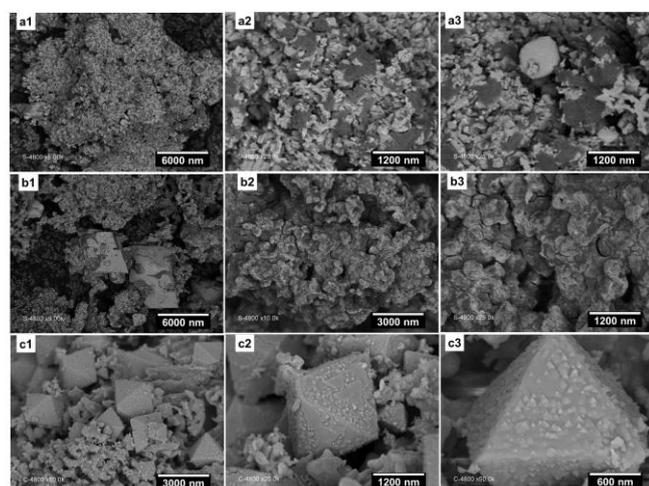
**Figure 2.** Backscattered SEM images of the as-synthesized materials. (a1-a3) PANI-Ni, (b1-b3) PANI-Co, (c1-c3) PANI-NiCo.
